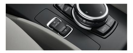
To complement the default COMFORT setting, the BMW i3 also offers two special driving modes to help you extend driving range. To select the required driving mode, press the driving experience switch until you see ECO PRO or ECO PRO+ in the display.
